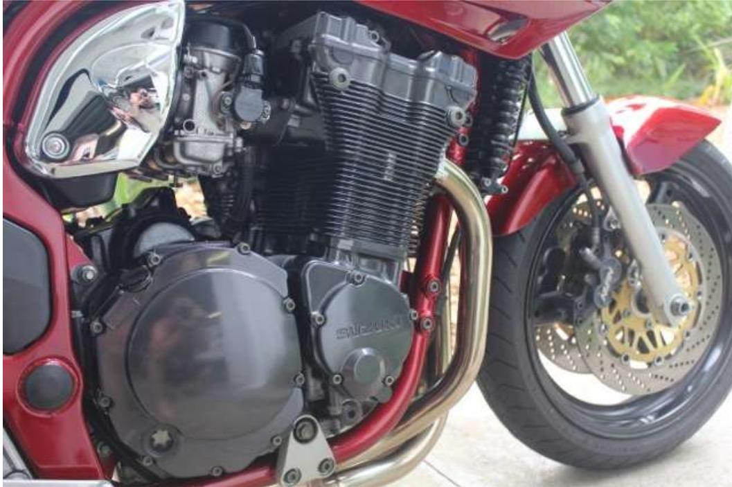
Photo #11 & #12 - Bandit 1200 engine is effectively the same engine as the GSXR1100. Exactly the same external dimensions. Bandit engine is 1157cc whereas the GSXR1100 started as 1052 and the last was 1127cc. Bandit runs different cams and slightly lower compression. The GSXR's put out more horsepower but due to the Bandit's torque it's a stump puller. The standard 1200 engine puts out about 95hp, but it doesn't take a massive amount of money to get 120>130hp or more out of this engine .
