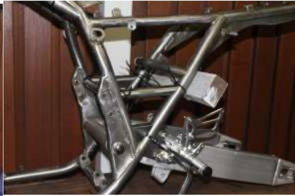
Photo #8 - Rear Set Mounts to be welded.
