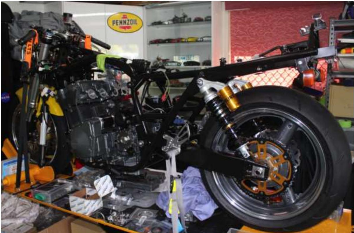
Head torqued down, GSXR1100 cams, Ape cam chain and slotted sprockets in place. Valve rockers adjusted and rocker cover bolted on.
