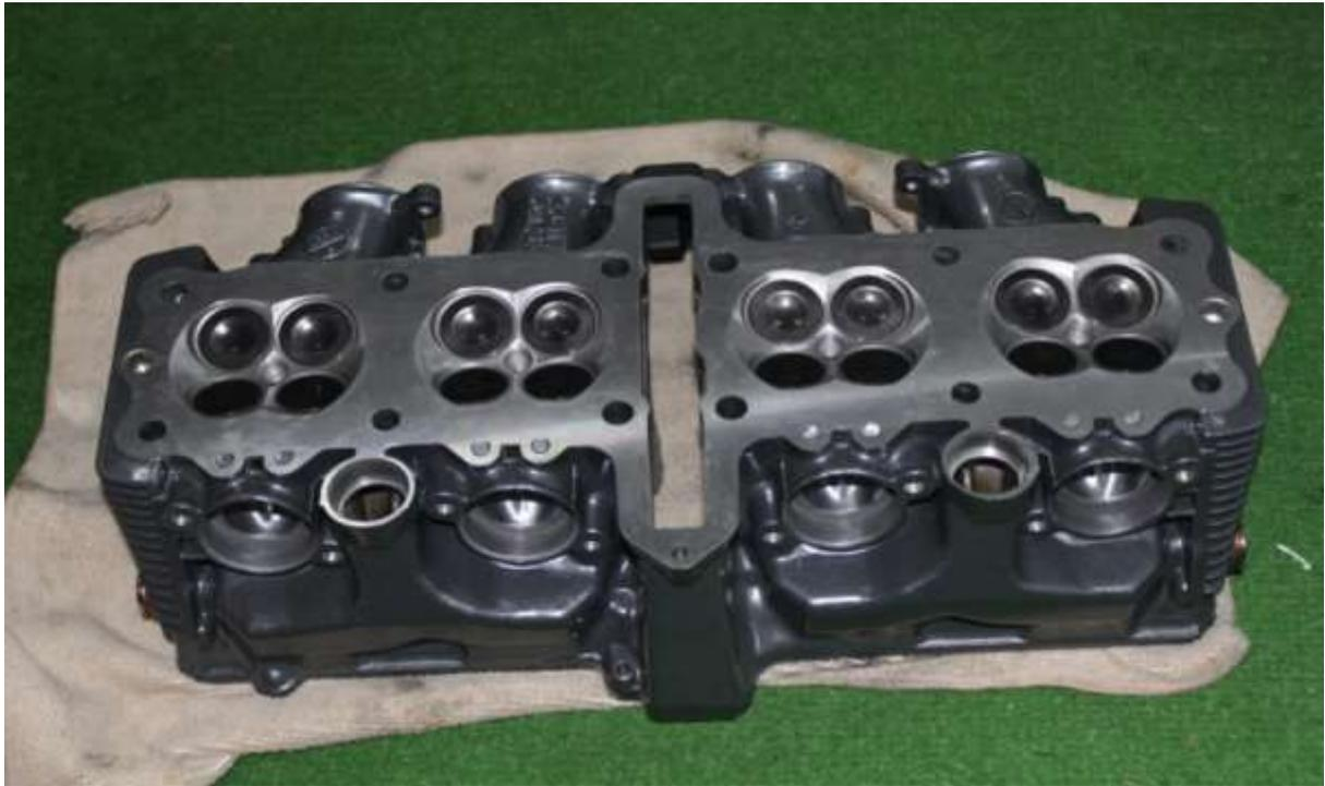
Coming together now. Barrels had light hone done by Steve at Myers. New rings fitted to pistons – Standard bore. Head lightly port and polished. Engine is back in the frame. Not quite complete.
