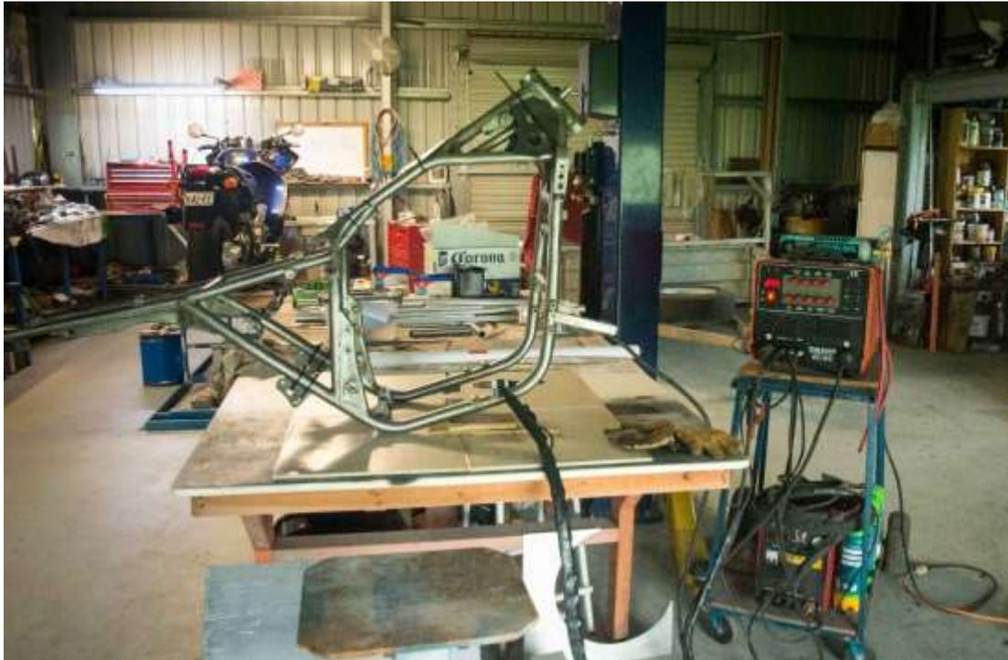
Now Gary, as a good aviation person is worried about rust so he gives me a Katana frame completely covered in Lanoline – to weld !! After sandblasting and two washes with pure acetone, I still can't get the weld working properly, never realised how good Lanoline is. LOL.
